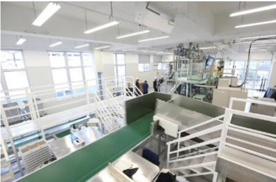
This Novetex Upcycling Factory will eventually have 3 production lines, each capable of producing one ton of recycled fibres a day from post-consumer textiles.
